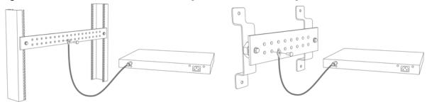
4 The grounding terminal of the server rack or on-site grounding terminal must also be grounded and connected to the building's main grounding electrode. Make sure the grounding terminal is connected to the buildings grounding electrode and has an earth resistance of less than 10 ohms, or according to your country's electrical regulations.
