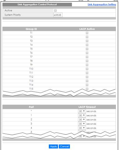
Figure 131 Advanced Application > Link Aggregation > Link Aggregation Setting > LACP
