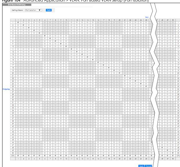
Figure 104 Advanced Application > VLAN: Port Based VLAN Setup (Port Isolation)
