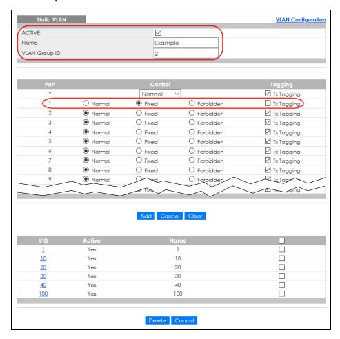
Note: The **VLAN Group ID** field in this screen and the **VID** field in the **IP Setup** screen refer to the same VLAN ID.
