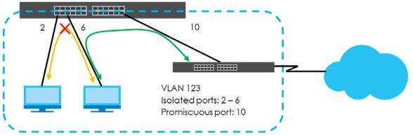
Note: Make sure you keep at least one port in the promiscuous port list for a VLAN with VLAN Isolation enabled. Otherwise, this VLAN is blocked from the whole network.
