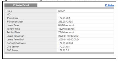
Table 19 Basic Setting > IP Setup > IP Status Details: DHCP
