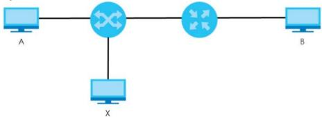
In this example, computer **B** tries to establish a connection with computer **A**. Computer **X** is in the same broadcast domain as computer **A** and intercepts the ARP request for computer **A**. Then, computer **X** does the following things:
