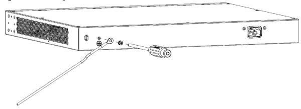
Attach the other end of the ground cable to a grounding bar located on the rack where you install the Switch or to an on-site grounding terminal.
