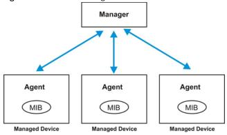
An SNMP managed network consists of two main components: agents and a manager.
