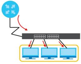
Figure 108 Static Multicast Forwarding to a Single Port
