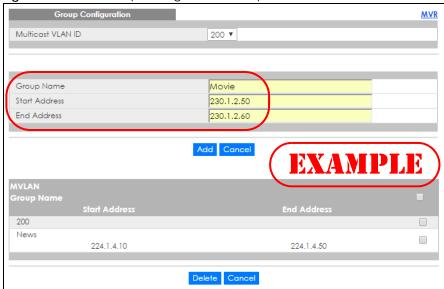
Figure 169 MVR Group Configuration Example-2
