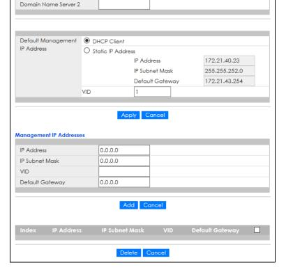
Table 20 Basic Setting > IP Setup > IP Configuration
