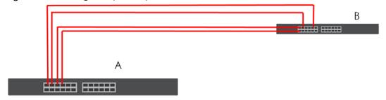
2 Configure static trunking – Click Advanced Application > Link Aggregation > Link Aggregation Setting. In this screen activate trunk group T1, select the traffic distribution algorithm used by this group and select the ports that should belong to this group as shown in the figure below. Click Apply when you are done.
