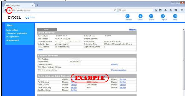
Figure 283 Example: Lock Denoting a Secure Connection
