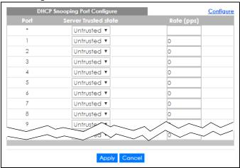
Table 109 Advanced Application > IP Source Guard > IPv4 Source Guard Setup > DHCP Snooping > Configure > Port
