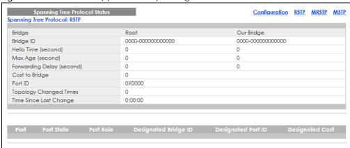
This screen differs depending on which STP mode (RSTP, MRSTP or MSTP) you configure on the Switch. This screen is described in detail in the section that follows the configuration section for each STP mode. Click **Configuration** to activate one of the STP standards on the Switch.
