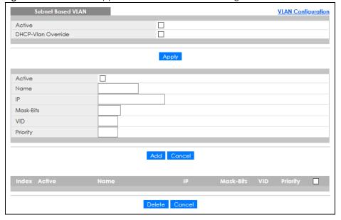
Table 44 Advanced Application > VLAN > VLAN Configuration > Subnet Based VLAN Setup
