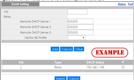
Figure 249 DHCP Relay for Two VLANs Configuration Example
