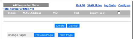
Table 112 Advanced Application > IP Source Guard > IPv4 Source Guard Setup > ARP Inspection Status
