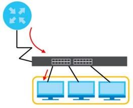
Figure 109 Static Multicast Forwarding to Multiple Ports
